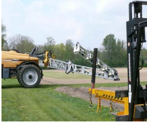
Fig.8: Moving of the outer boom section because of getting in contact with obstacle.
