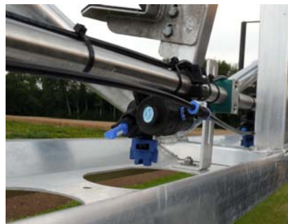
Fig.7: Nozzle station at the boom.
