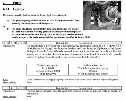
Fig. 3 Pump capacity
