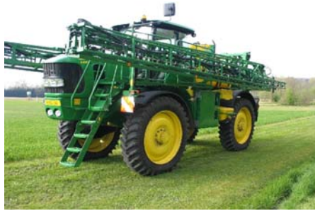
Fig.4: Left sprayer side with lateral folded boom and ascent to the drivers cabin.
