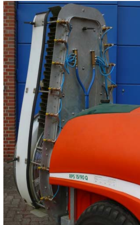
Fig.8: Axial fan „90 Q“ with 900 mm rotor
