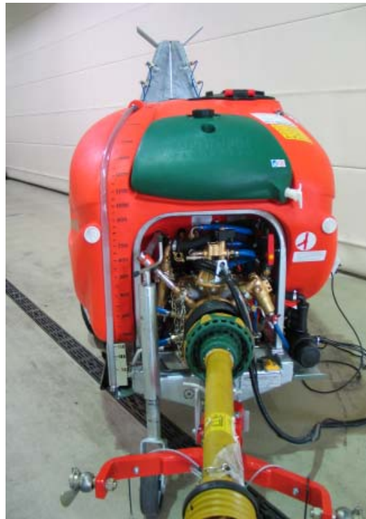
Fig.4: Front side with draw bar, pump, suction filter and front tank contents indicator
