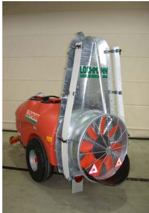
Fig.6: Axial fan „80 Q“ with 800 mm rotor and air intake from rear
