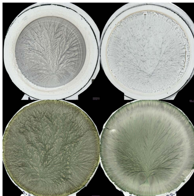
Fig. 1 Patterns from cupric chloride crystallization with above PVP-700 (left) and PVP-40 (right) and below milk protein concentrate (left) and whey protein concentrate (right) as additives.
