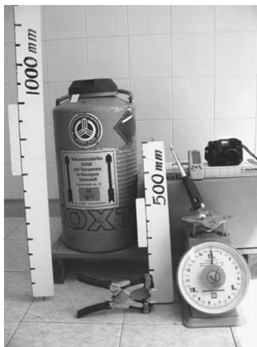
Figure 3 Equipment for collecting somatic cell samples: large ruler, transportation cryo tank, tagger, small ruler, pipette, global positioning system device, scale and digital camera (left to right).
